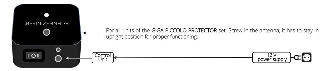
One unit of the GIGA PICCOLO PROTECTOR set is labeled as **MASTER**. The **CONTROL UNIT** will be connected to the GIGA PICCOLO PROTECTOR and the **12V power supply** will be connected to the CONTROL UNIT.
