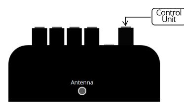
Screw in the big antenna (alternatively due to lack of space the small version); it has to stay in upright position for proper functioning.
